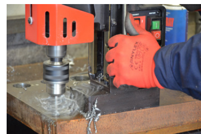
Drilling capacity up to 16 mm (0.63") - with cylindrical shank twist drill in use Drilling capacity up to 23 mm (0.91") - with MT2 shank twist drill in use
