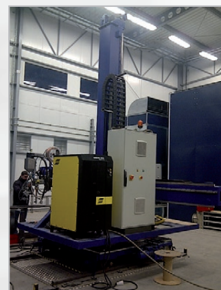
Half Gantry Beam and Tank Welding System C&B type WA with LINCOLN ELECTRIC PW AC/DC 1000 SD
