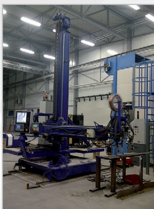
Standard Column & Boom with ESAB Aristo 1000 AC/DC
