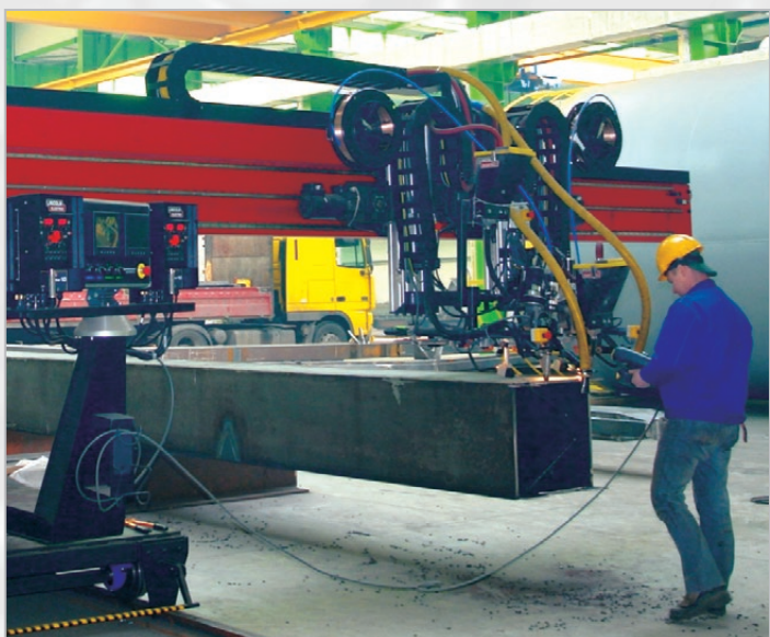
Standard Column & Boom with ESAB Aristo 1000 AC/DC
