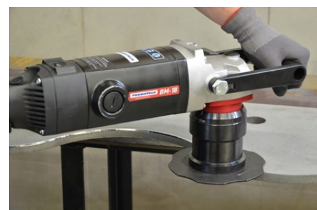
Rounding off curved edges
