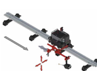
Motorized vertical slide OSK-0654-04-00-00-0
