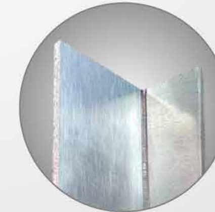
Aluminum-4.0mm T-type welding
