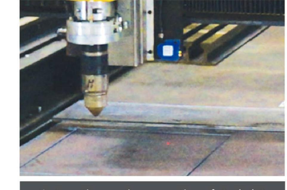
Automatic scanning correction of steel plate
